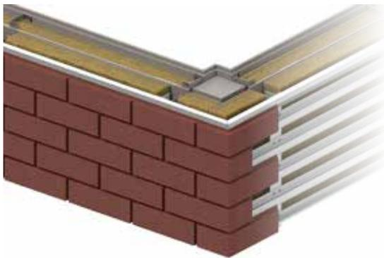
NaturAL-X brick tiles have an integrated rebate, consistently setting the vertical perp joint at 10mm. The corresponding 10mm horizontal bed joint is instantly created by the profiled top lip of the adjacent brick tile.
