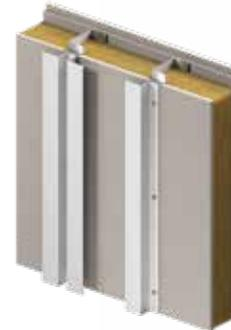
Aluminium support system suitable for rainscreen with a shallow cladding zone and no adjustability requirement.
