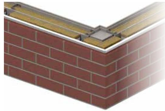
When installation is complete, simply injection point these joints with Parex Historic mortar to realise a classic clay brick finish.
