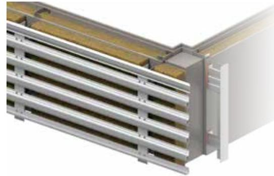
Horizontally affix middle rails to the vertical supports at 75mm increments, including a starter and top rail in their respective locations.
